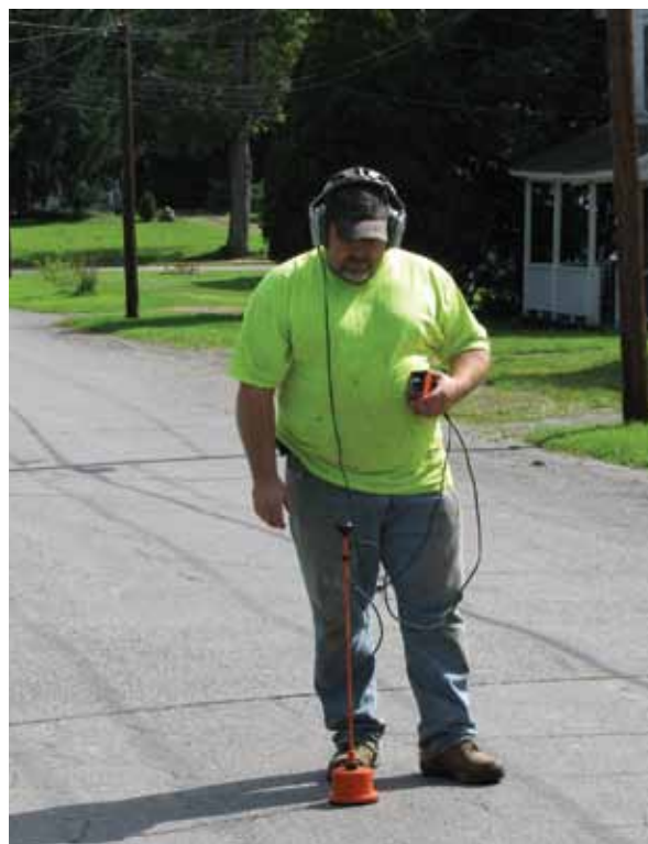
An active leak detection program is critical for reducing water loss.
